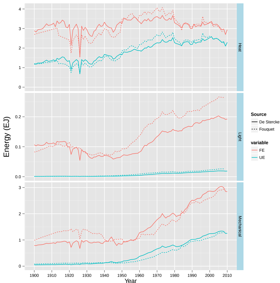
Figure 9: Comparison of total final energy and useful energy per use for the United Kingdom, between Fouquet (2008) and this study. The useful energy series have been estimated using the final-to-useful energy conversion efficiency model developed for the present study. Feedstocks (non-energy uses) are not shown in this graph. The scale on the vertical axis varies across panels.
